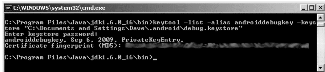
Figure 7-6. The keytool output for the list option (actual fingerprint smudged on purpose)
